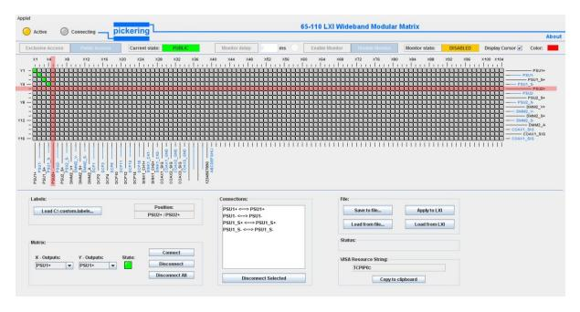
Figure 3. The soft front panel of the 65-110 can be accessed through the LXI configuration pages to either control or monitor the matrix settings. The LXI controller presents the matrix as a single entity, greatly simplifying the user understanding of the setting
