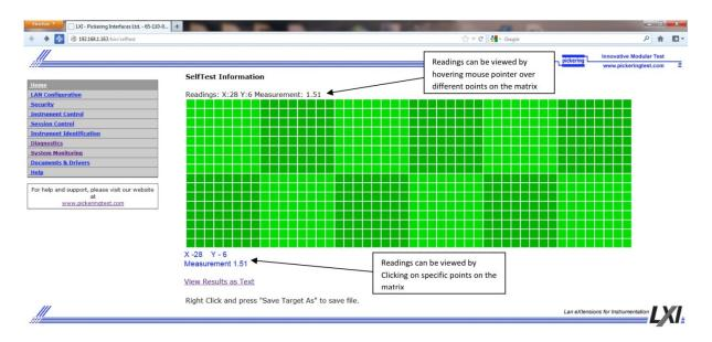
Figure 4 The web interface on 65-110 allows easy access to the self test facility through the standard LXI cofiguration pages.
