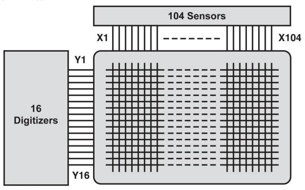
Figure 1. The CERN requirement requires a matrix to connect up to 104 analogue sources to up to 16 digitisers
